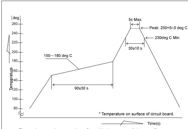
The products may be exposed to reflow soldering process of above profile up to two times.
